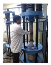
Test for Determining Creep Coefficient (In Compression)
