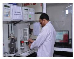
Mercury Intrusion Porosimeter is used to study the pore size distribution and porosity determination of aggregate, concrete and mortar
