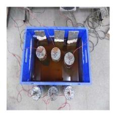
Accelerated Chloride Induced Corrosion Studies
