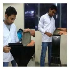
V-Funnel & L-Box Test for SCC
