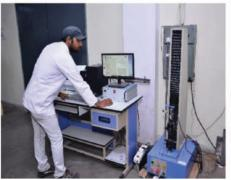
Tensile Testing of Steel Fibers
