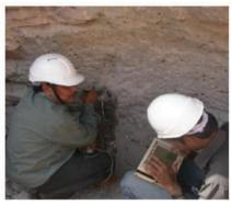
Pile Integrity Test of Prestressed Concrete Bridge
