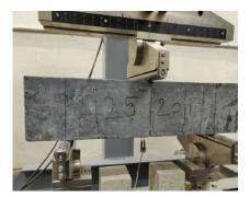
Testing of notched beam in progress for the study of fracture behaviour of High Strength Concrete
