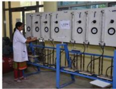
Water Permeability Testing on concrete samples
