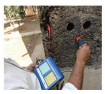
Half-cell Potential Measurement of Corrosion Damaged Structure
