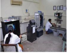
Strain Controlled Flexural Testing Machine-300kN for determination of flexural toughness of fiber reinforced concrete & crack mouth opening gauge for measurement and control of crack width
