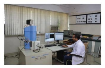
Scanning Electron Microscope with EDAX
