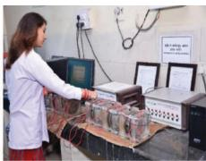
Rapid Chloride Penetrability Test for concrete samples to study the degree of penetrability of chloride ions
