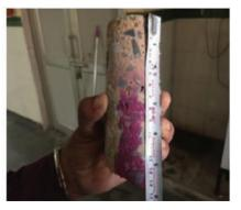
Carbonation depth being measured on freshly extracted core at site
