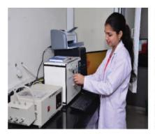
BET Apparatus for determining fineness of ultra-fine powder materials such as silica fume, metakaolin, ultrafine fly ash, ultrafine slag etc. has been procured and installed
