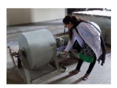
Abrasion Value Test for Aggregate
