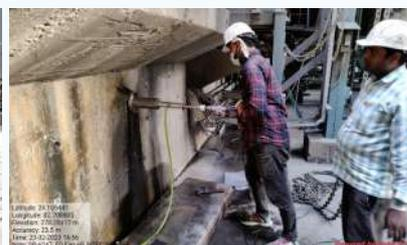
NCB Team carrying out Non-Destructive Testing at FD fan foundation structure at NTPC Singrauli
