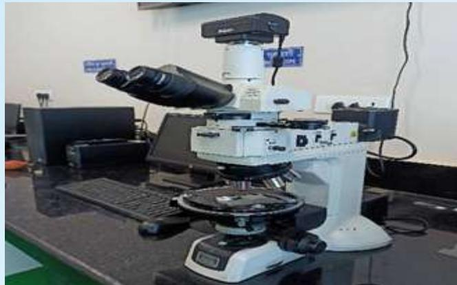
Polarizing Microscope, Make: NIKON Japan, Model: POL 100 LV
