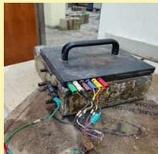
Measurement of corrosion rate using LPR
