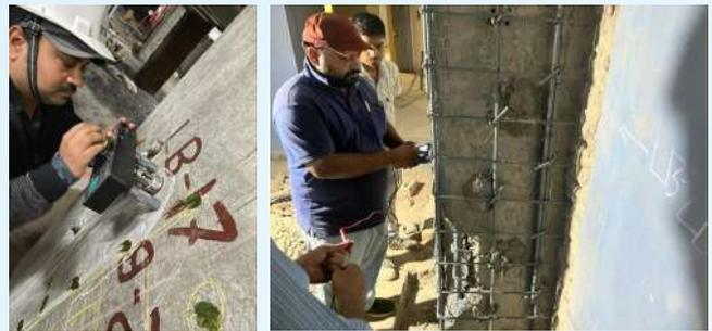
NCB Team carrying out Pull-off test on repaired columns and checking electrical continuity of installed anodes at NHAI site
