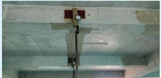
**Load testing with sand-filled bags in progress on the RGC slab structure**
