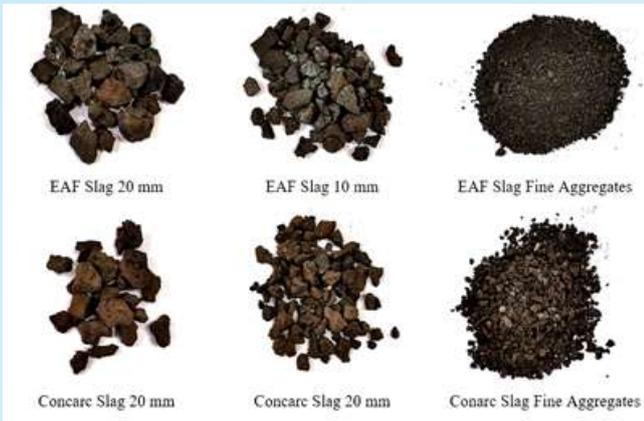
**EAF slag and Conarc slag – coarse as well as fine**
