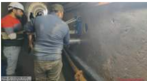
Concrete Core Extraction from the Dam Gallery Location of Teesta-V Dam
