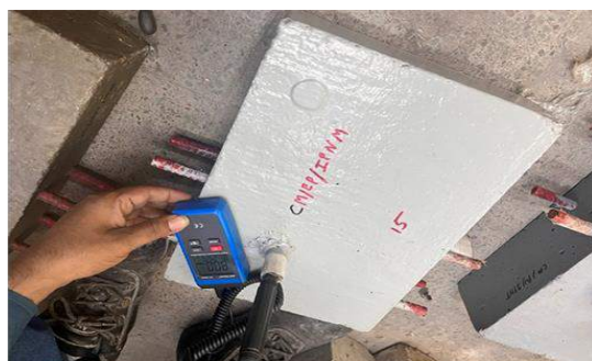
Testing of relative humidity in the coated concrete slabs as per ASTM F2170.
