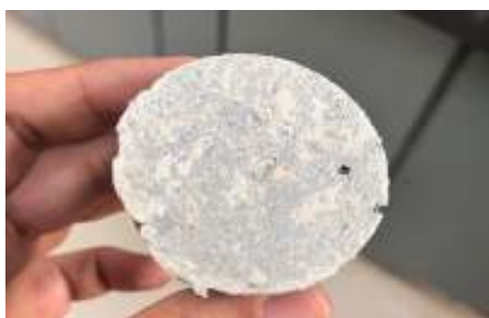
Coated concrete samples of dia 50mm after pull-off testing as per ASTM-C1583:2020
