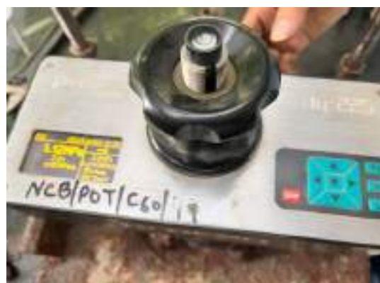
Pull-off adhesion test being done on coated concrete specimen
