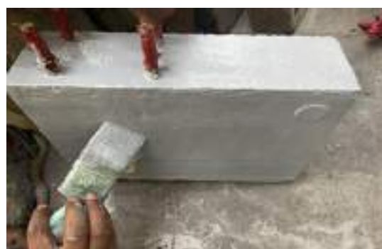
Application of coating material on concrete slab samples by brush.
