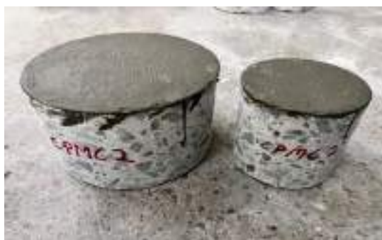
Prepared/coated concrete cylindrical samples of dia 100mm and 150mm before testing.
