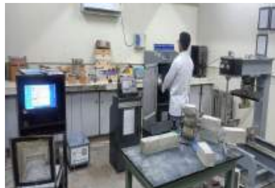
Strain Controlled Flexural Testing Machine for determination of flexural toughness of concrete
