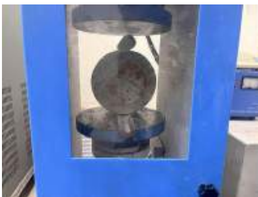
Coated concrete cylinder specimen being broken into two half for Depth of Water Penetration measurement
