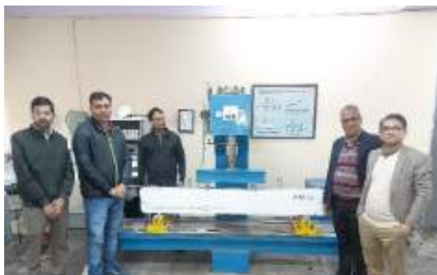
Test set up for testing of beam in four-point bend test
