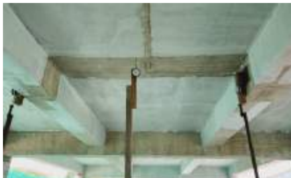
Placement of dial gauges below slab and beams for recording deflections during load test
