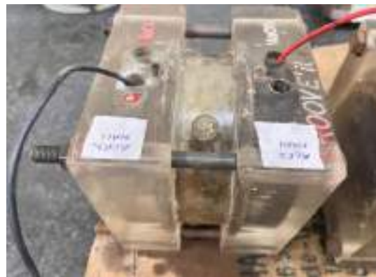
NT Build 492 Testing being done on coated concrete specimen
