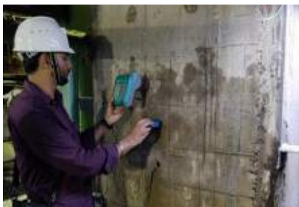
Half Cell Potential Measured Column at NTPC, Korba
