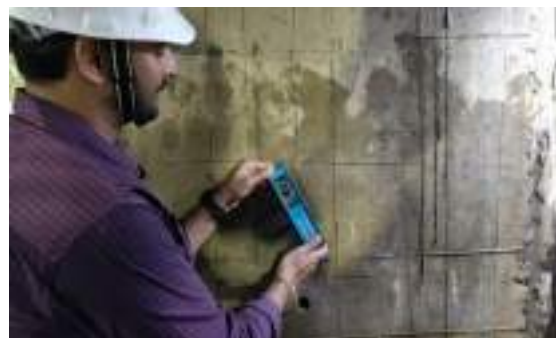
Electrical Resistivity Measured on TG Column at NTPC, Korba
