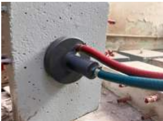
Air Permeability Testing being done on coated concrete slab specimen
