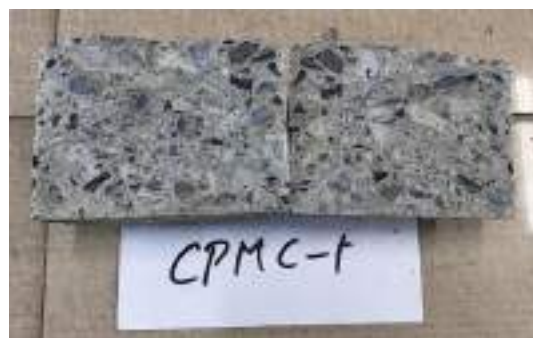
Splited concrete cylindrical samples of dia 150mm after water penetration testing as per IS 516: Part2/Sec1: 2018.
