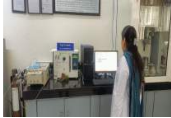
Surface Area determination of cementitious Materials through BET apparatus
