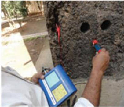
Half-cell Potential Measurement of Corrosion Damaged Structure
