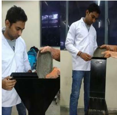
V-Funnel & L-Box Test for SCC
