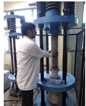
Test for Determining Creep Coefficient (In Compression)
