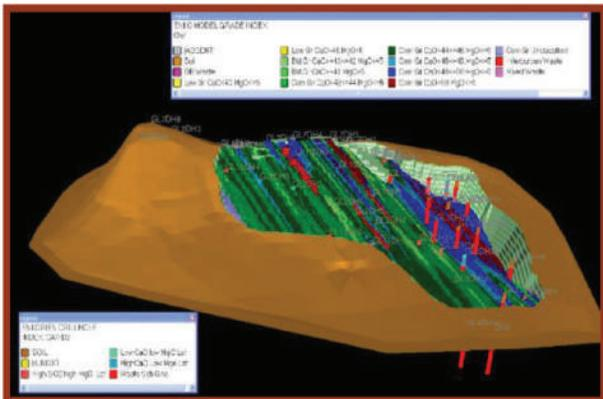
**3-D Ore Body Model of LS Grade Distribution within Conceptualized Pit**
