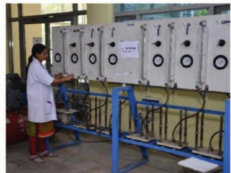
Water Permeability Testing on concrete samples
