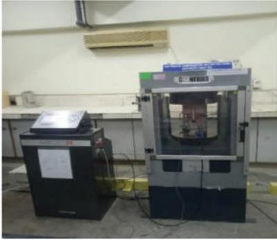
Testing for Stress Strain curve in progress for High Strength Concrete
