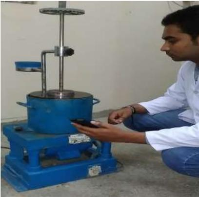
Workability Measurement of Roller Compacted Concrete
