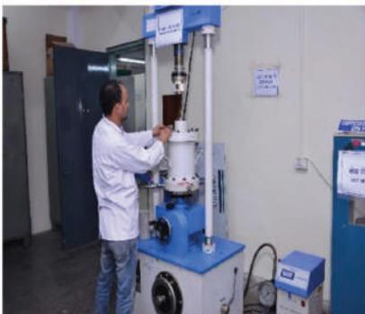
Confined Compressive strength of Concrete and Rock Specimens
