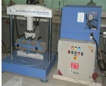
Concrete Fibre reinforced Beams (In Flexure)
