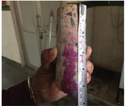
Carbonation depth being measured on freshly extracted core at site
