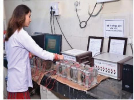
Rapid Chloride Penetrability Test for concrete samples to study the degree of penetrability of chloride ions
