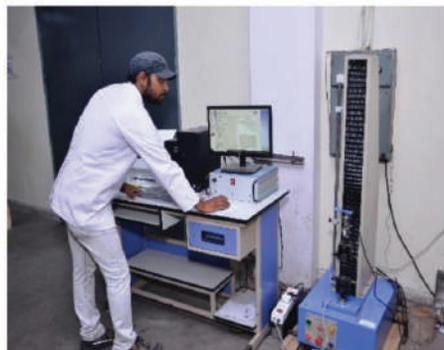
Tensile Testing of Steel Fibers
