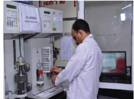
Mercury Intrusion Porosimeter is used to study the pore size distribution and porosity determination of aggregate, concrete and mortar
