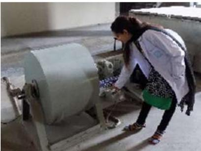
Abrasion Value Test for Aggregate
