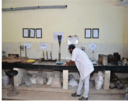
Marsh Cone Test for ultra-fine cement to study the flow ability of cement
