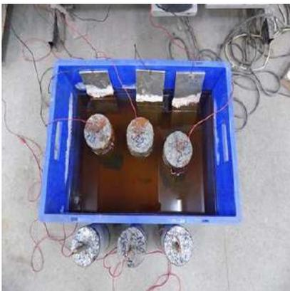
Accelerated Chloride Induced Corrosion Studies
