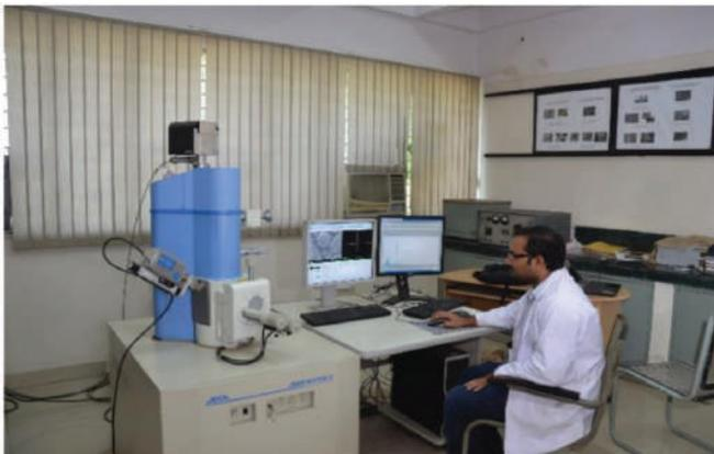
**Scanning Electron Microscope with EDAX**
