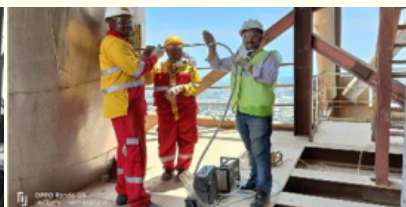
Monitoring of PM & Gaseous Emissions at Kiln Stack
