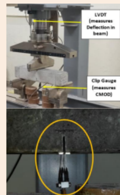
Experimental setup for evaluation of fracture parameters
