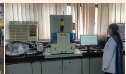
Mercury Intrusion Porosity equipment for checking porosity of concrete
