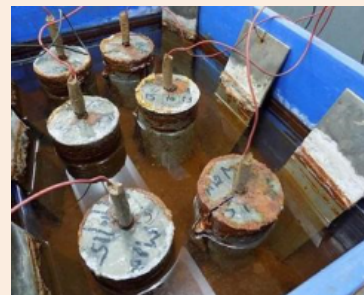
Accelerated Corrosion Test
