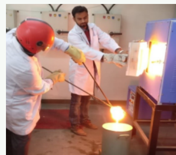
Development of synthetic slag in laboratory
