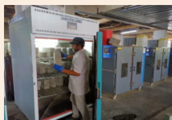
Hardened Concrete Sample - Accelerated Carbonation
