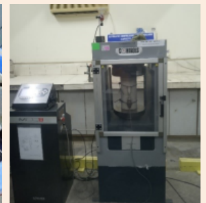
Test setup for Stress-Strain study of concrete under Strain controlled mode
