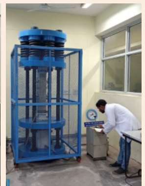
Creep Testing Arrangement for Ultra-High Performance Concrete
