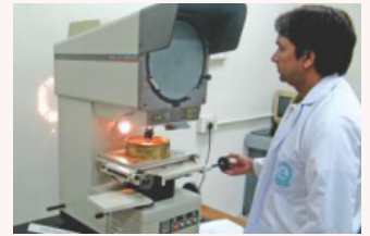
Calibration of Sieve at Profile Projector
