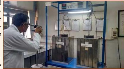
During the calibration procedure, it has to be ensured that the stability of the temperature is maintained. The whole procedure is repeated over the desired calibration range of the temperature.
