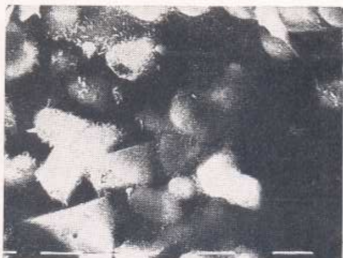
Plate II. Well developed alite and belite in yellow clinker
